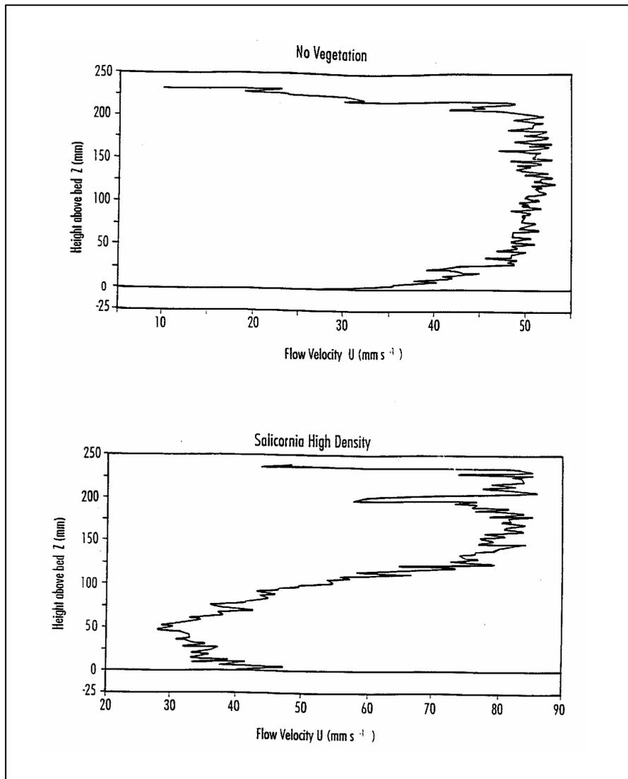
**Figure A1.5** Velocity profiles over a bare mudflat (top) and within saltmarsh vegetation (bottom) (from Toft et. al, 1995)
