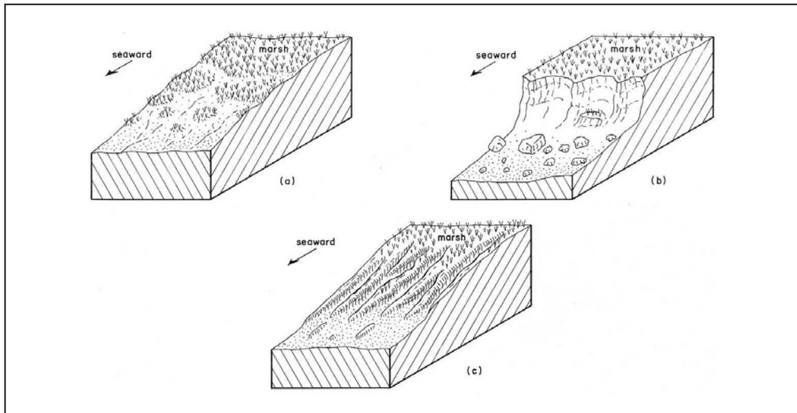
**Figure A1.2** High tide morphologies along a muddy shoreline: (a) smooth transition from mudflat to saltmarsh, (b) bold marsh cliff, (c) marsh ramp with wave-scoured spurs and furrows (after Allen, 1993)
