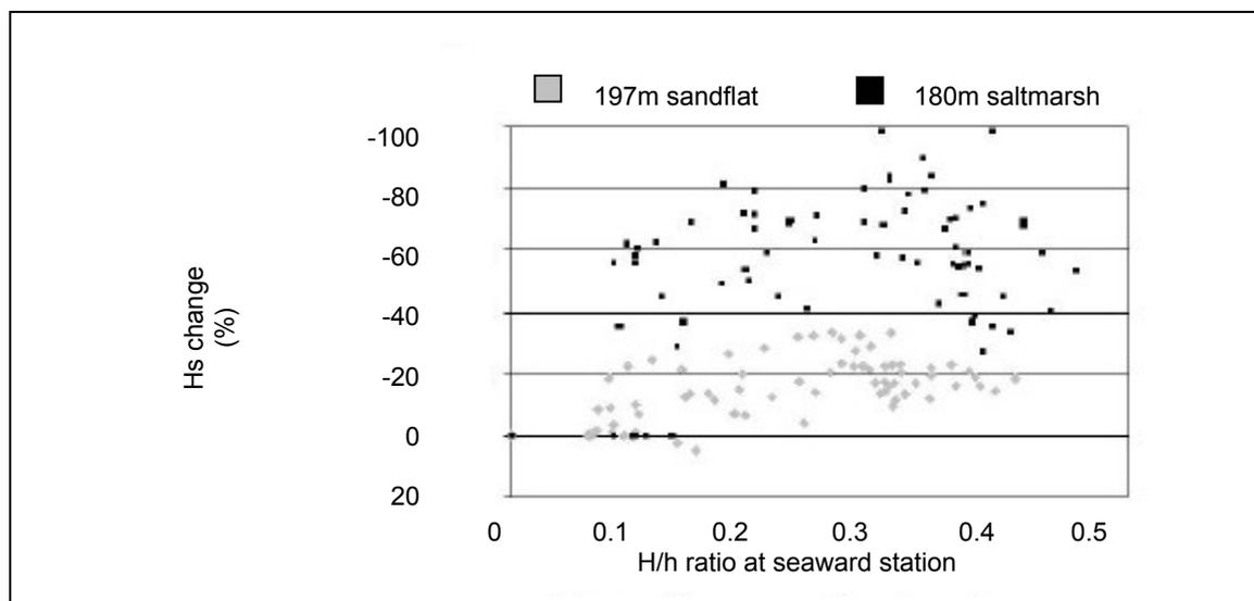
**Figure A1.10** Relationship between wave energy attenuation and water depth for the sand flat and saltmarsh areas at Stiffkey, north Norfolk (from Möller et al., 1999)
