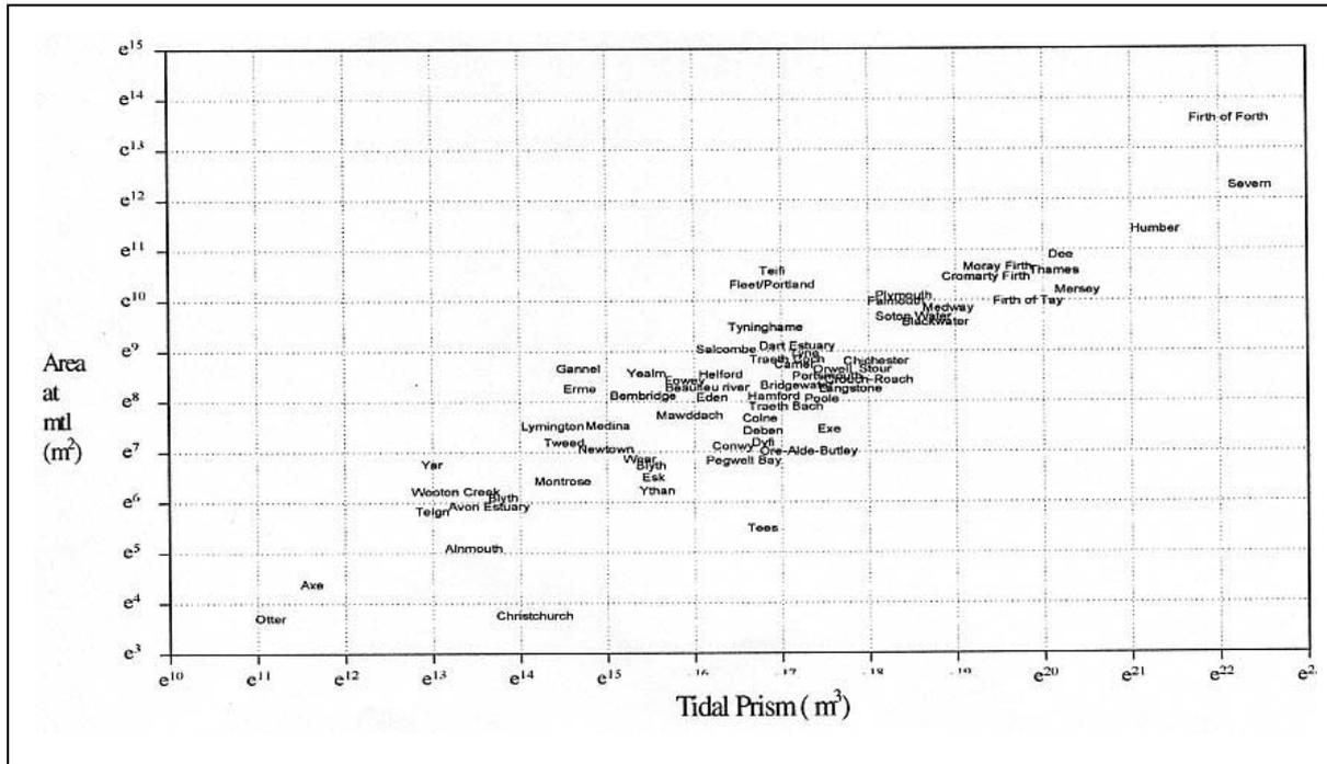
**Figure A1.1** Plot of tidal prism against cross sectional area (mean tide level) for United Kingdom estuaries (after Townend *et al.*, 2000)
