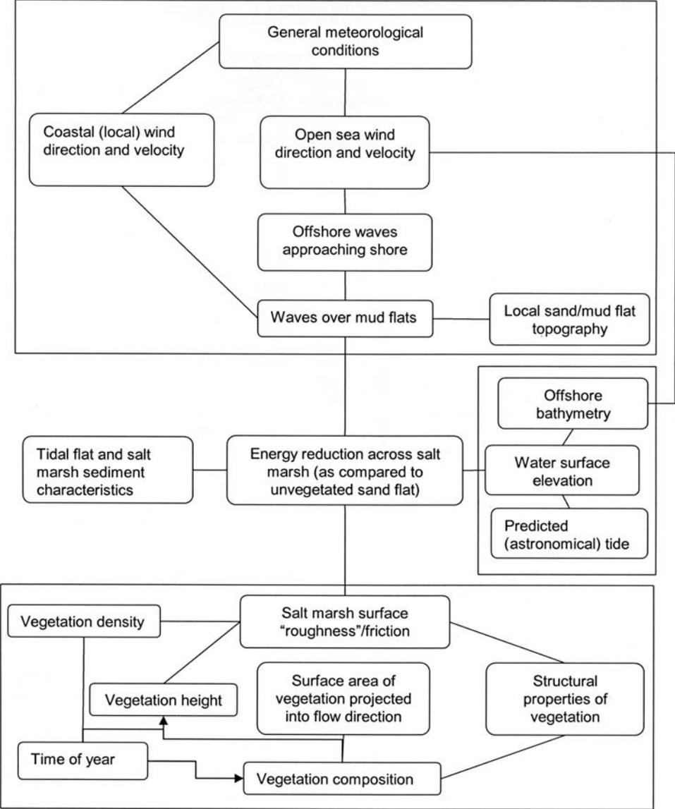
**Figure A1.9 Factors influencing wave energy dissipation over saltmarshes (from Möller et al., 2002)**
