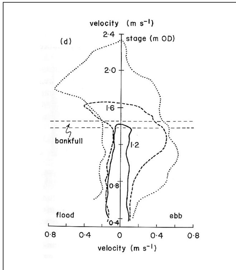
**Figure A1.7** Example of a velocity-stage curve measured within creeks for undermarsh (solid line), bankfull (dashed line) and overmarsh tides (dotted line) (after Allen, 2000)
