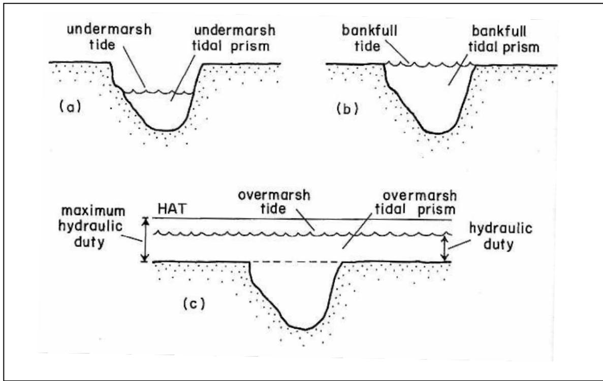
**Figure A1.6** A classification of tides and tidal prisms affecting saltmarshes; hydraulic duty is the height difference between the saltmarsh surface and the level of high water (after Allen, 2000)
