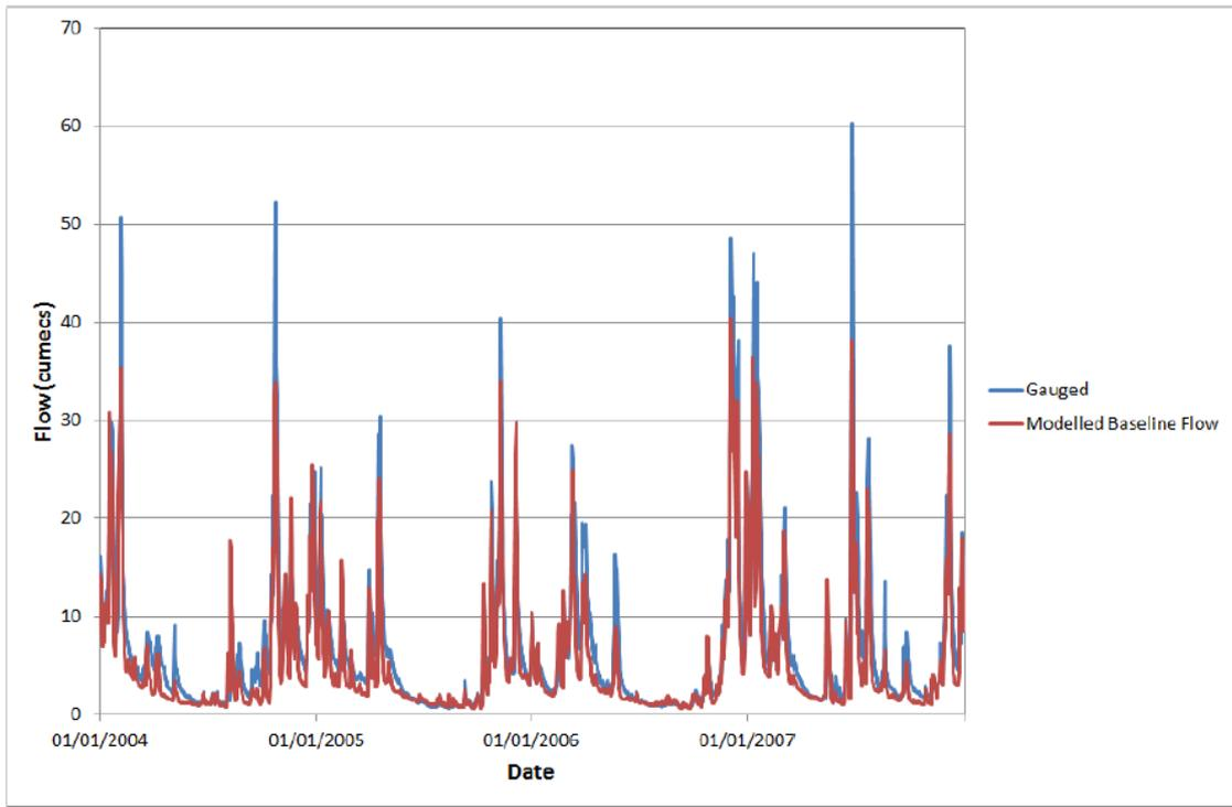
**Figure 5: CERF model daily flows compared with observed flows over sample period at Pont-y-Cambwyll**
