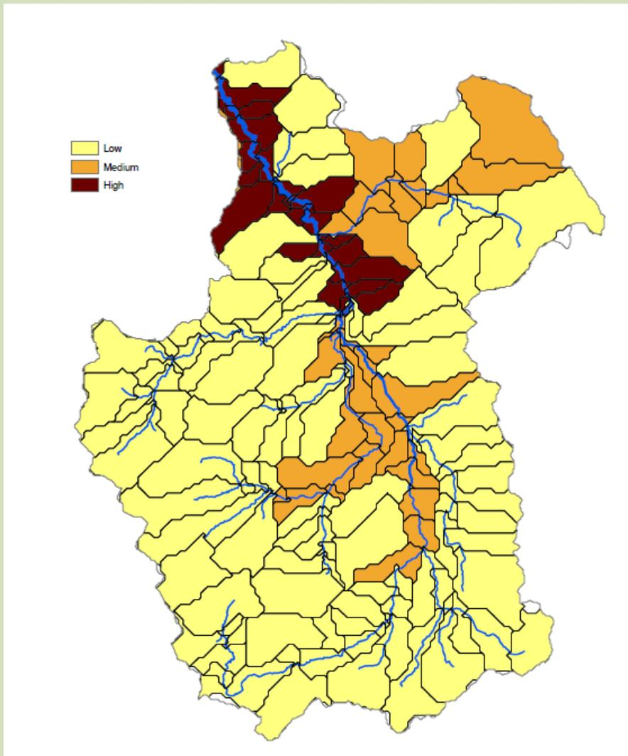
**Figure 4: Fine sediment supply within the Clwyd catchment**
