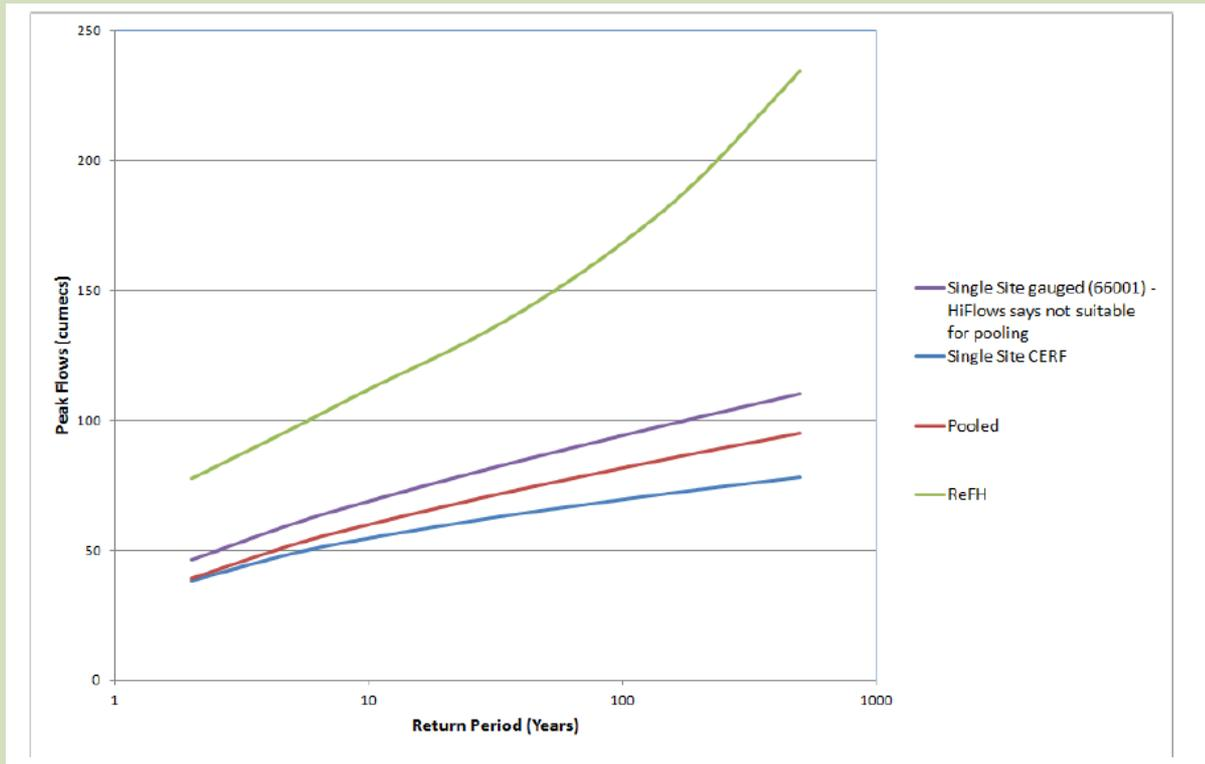
**Figure 2: Flood frequency curves using the model and comparison with ReFH and FEH statistical parameters**
