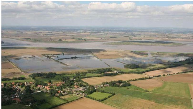
**Figure 1.6 Alkborough Flats managed realignment – breach to the right
