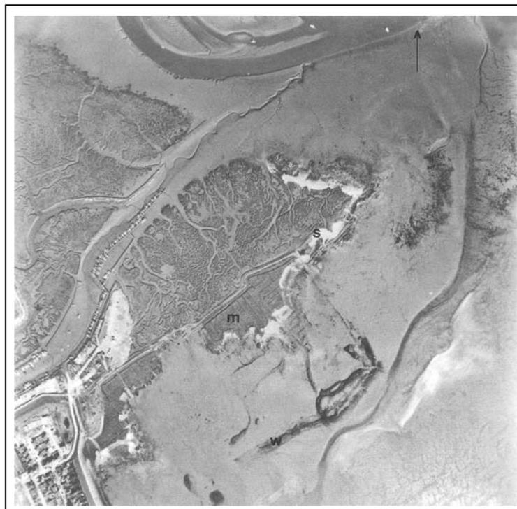
**Figure C.4** Aerial photograph of part of Canvey Island, Essex, showing severely eroded area of marsh formed after the breaching of the surround sea wall in 1881 (from Toft et al., 1995)
